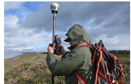
John Herrera uses a Trimble R10 Real Time Kinematic GPS units at Lanphere.
